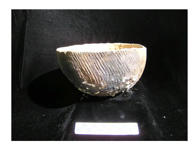
**Replica vessel 3, used to boil water for approxi**mately two hours, spalled to the point of failure.
